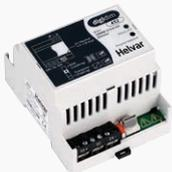
1-10V / DSI Convertor. Connect and dim analogue or legacy digital dimmable ballasts. Integral 16A relay for analogue dimming. DIN rail mounting.
