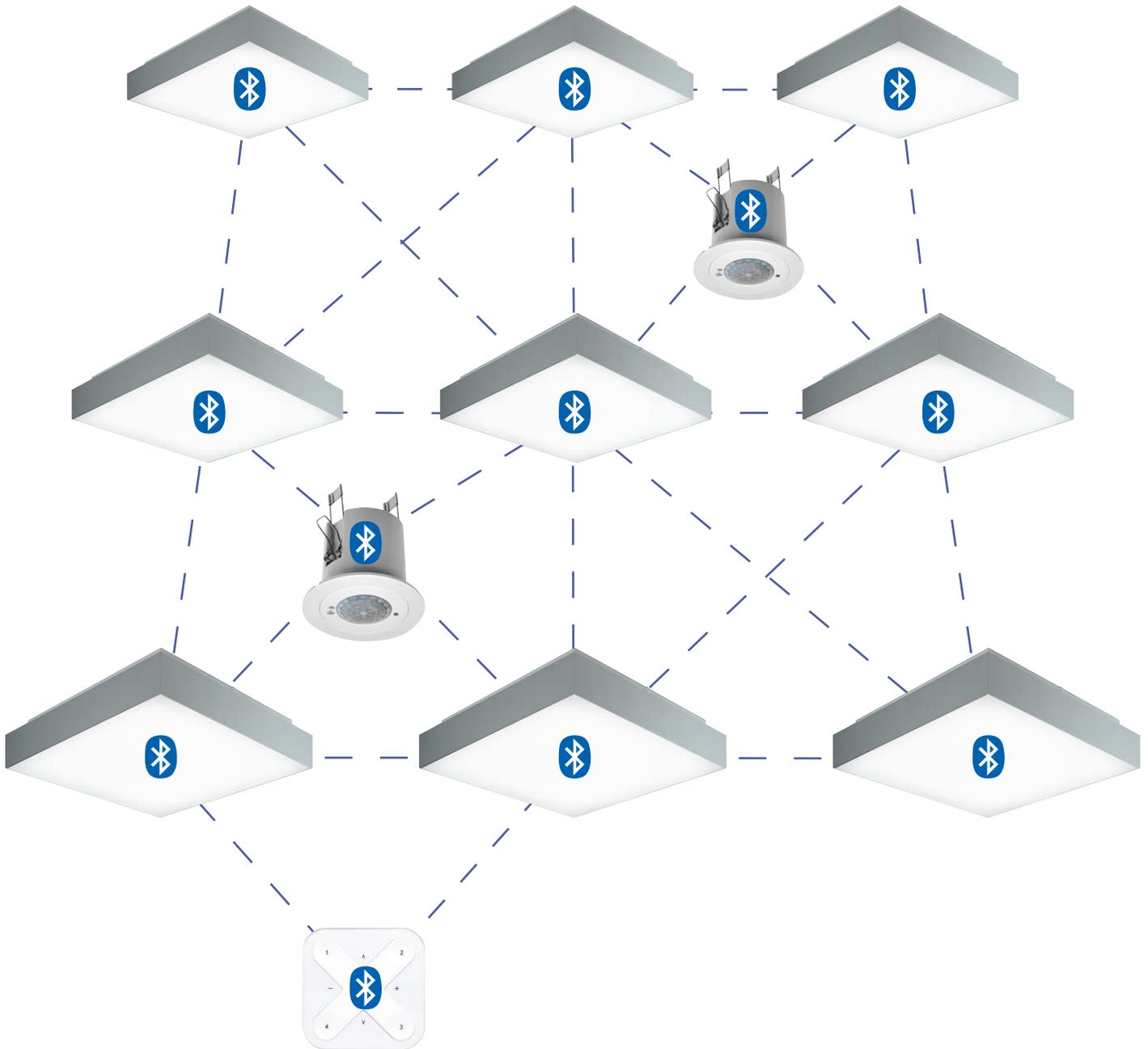
Light fittings and sensors only require a mains connection. Switches and scene plates are either wireless and batteryless or contain a long life Lithium coin battery - in either case no wiring is required.
